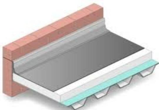
The deck should be installed or laid with an even fall sufficient to allow water to drain to rainwater outlets. Code of practice recommends a minimum finished fall of 1:80.
